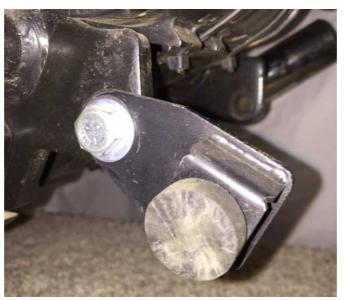
Install on OUTSIDE of tab as shown. If mounted to the inside it can affect the kickstand alignment and clearance to the mufflers. Remove rubber pad from stock mufflers and install on bracket.
