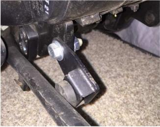
Align stop bracket and kickstand. Complete final tightening. You can affect the kick stand distance from the muffler by rotating the kickstand stop bracket clockwise/counterclockwise.
