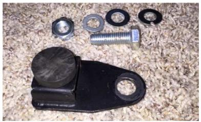
This is the Thruxton and "Mag Wheel" Bonneville kickstand stop bracket and hardware provided with your exhaust kit. It is shown with the rubber kickstand stop (from your stock muffler) already installed.
